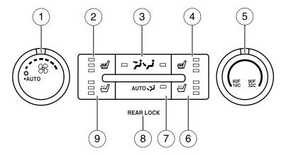
1. **Fan control:** Turn to select the desired fan speed or choose the following.
